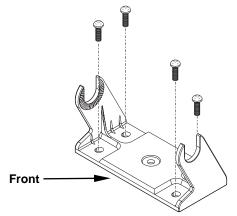
Install the gimbal bracket. Orient the bracket so the arms slope toward the front of your unit.
